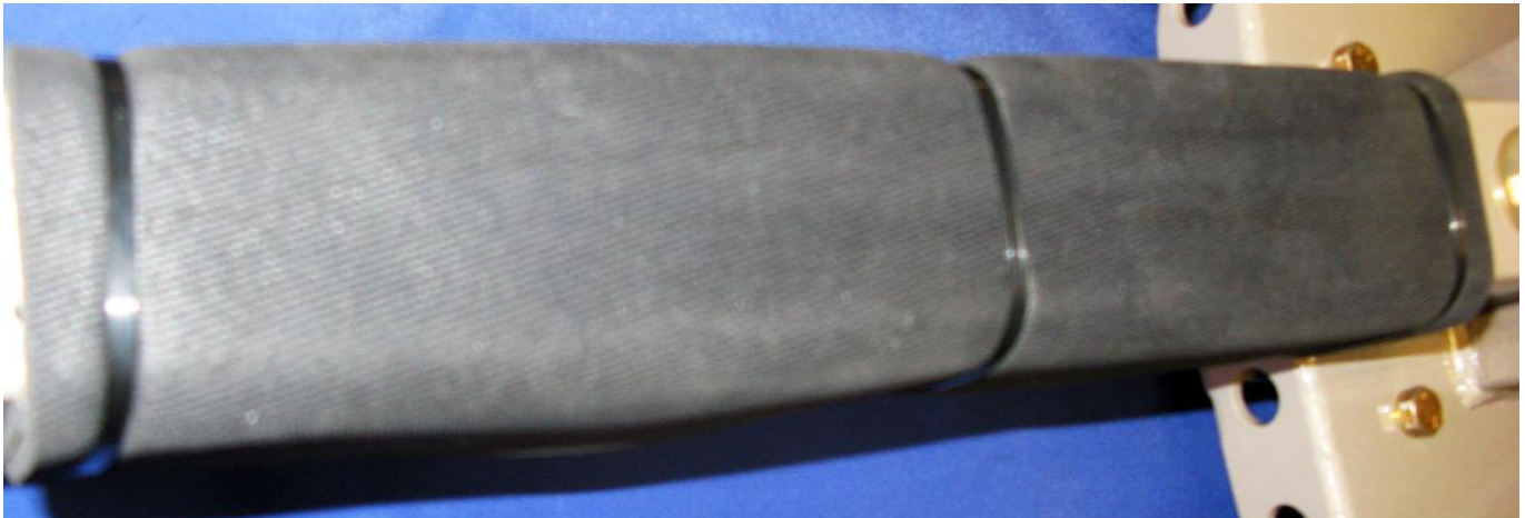
Photo – Placement of Zip-Ties for outer Foam Wrap on Main Root Tube
