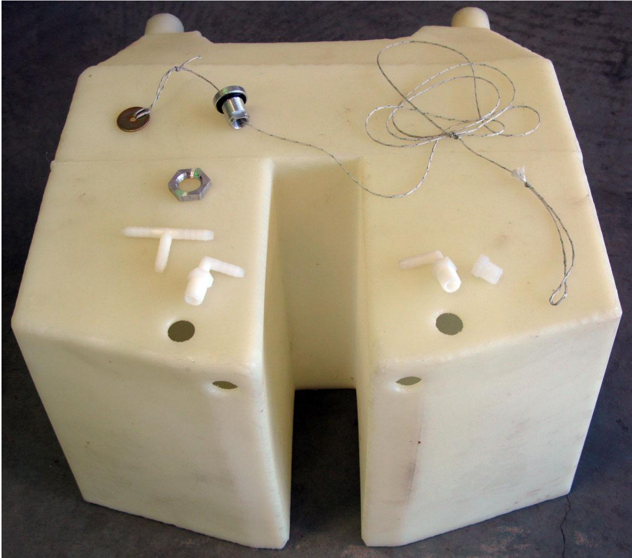
Photo – Fuel Tank, Bulkhead Fitting, Fuel Line Connectors
