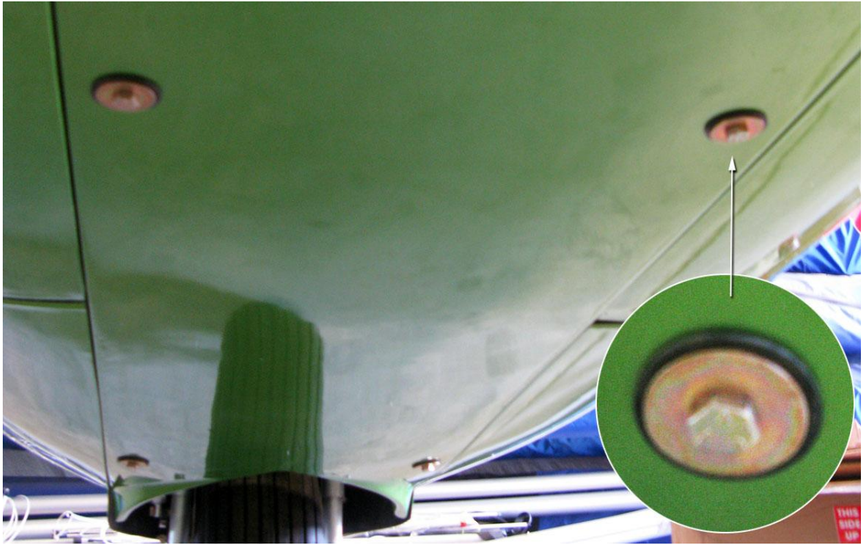
Photo: Bottom View of Belly Pan Attached to Root Tube Fairing Brackets
