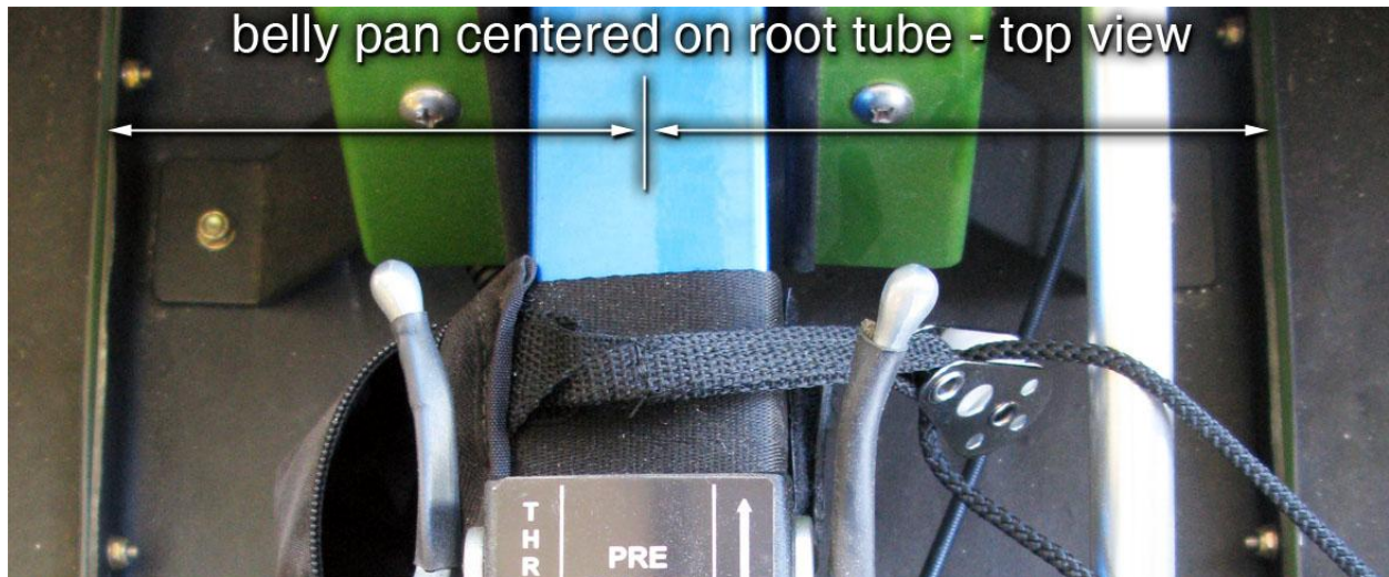
Photo: Fairing Belly Pan section centered on Root Tube of trike frame
