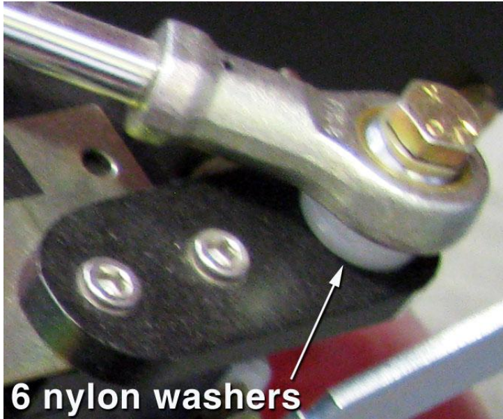
Photo – Bolt and washer assembly at rear of Steering Stabilizer
