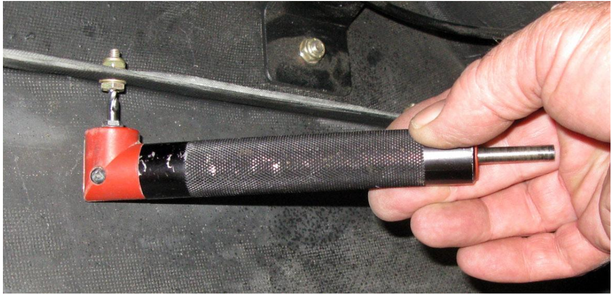
Photo: Example of small Angle Drill for drilling Front Fairing Section to Belly Pan Junction
