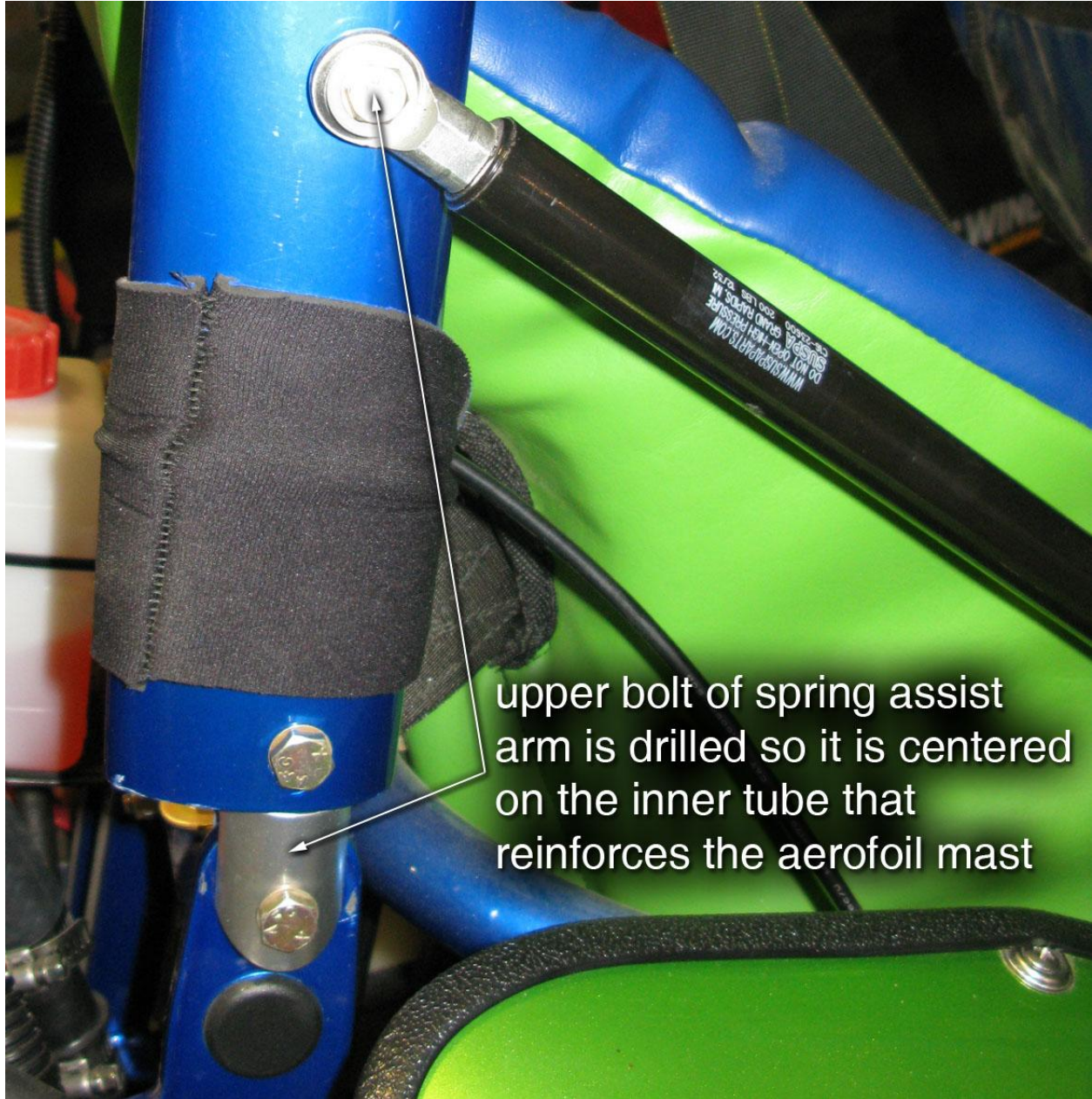
Photo: Locating bolt hole location on upper end of Spring Assist arm
