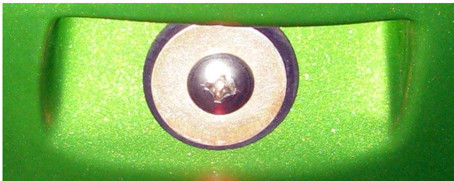
Photo: Bolt with Metal and Rubber Washers attached to nose of Fairing
