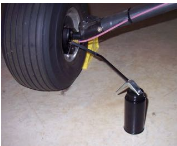
Brake fluid pump connected to bleeder valve with 1/4" tubing
