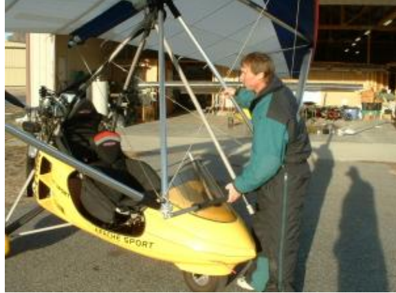
Figure 9: Lift Wing into Position
