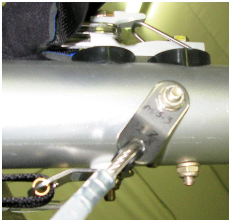
8. Attach the rear Flying Wires to the keel by placing a thick washer on the AN4-27A bolt, then place the metal tang of the right-side rear flying wire on the bolt, then add a white WN14 Nylon washer, then insert this bolt assembly through the right side of the keel.
