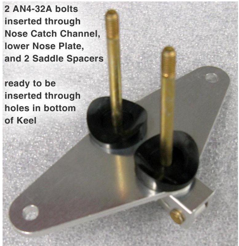
Photo: Attaching Top Nose Plate to Keel
