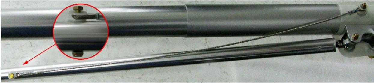
9. Attach the hardware for connecting the Cross Bar to the Channel Bracket. The Cross Bar will not be attached to this assembly until later, when the sail is added to the airframe. For now, attach the hardware so it can be used later when needed to attach the Cross Bar.
