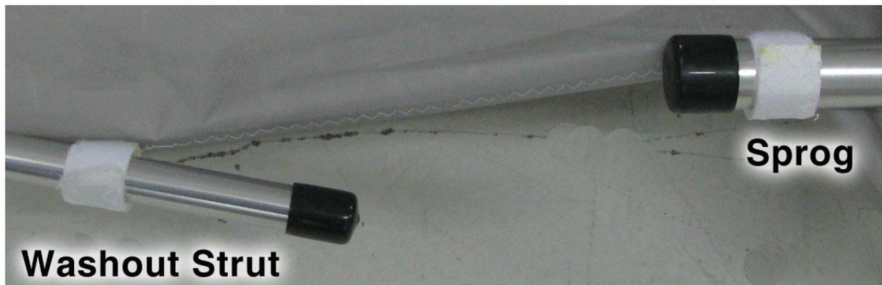
5. Pull the tip of the sail over the black cap at the end of the leading edges by pulling on the black strap, and be sure to set the yellow strap into the 1" wide slot at the end of the leading edge.
