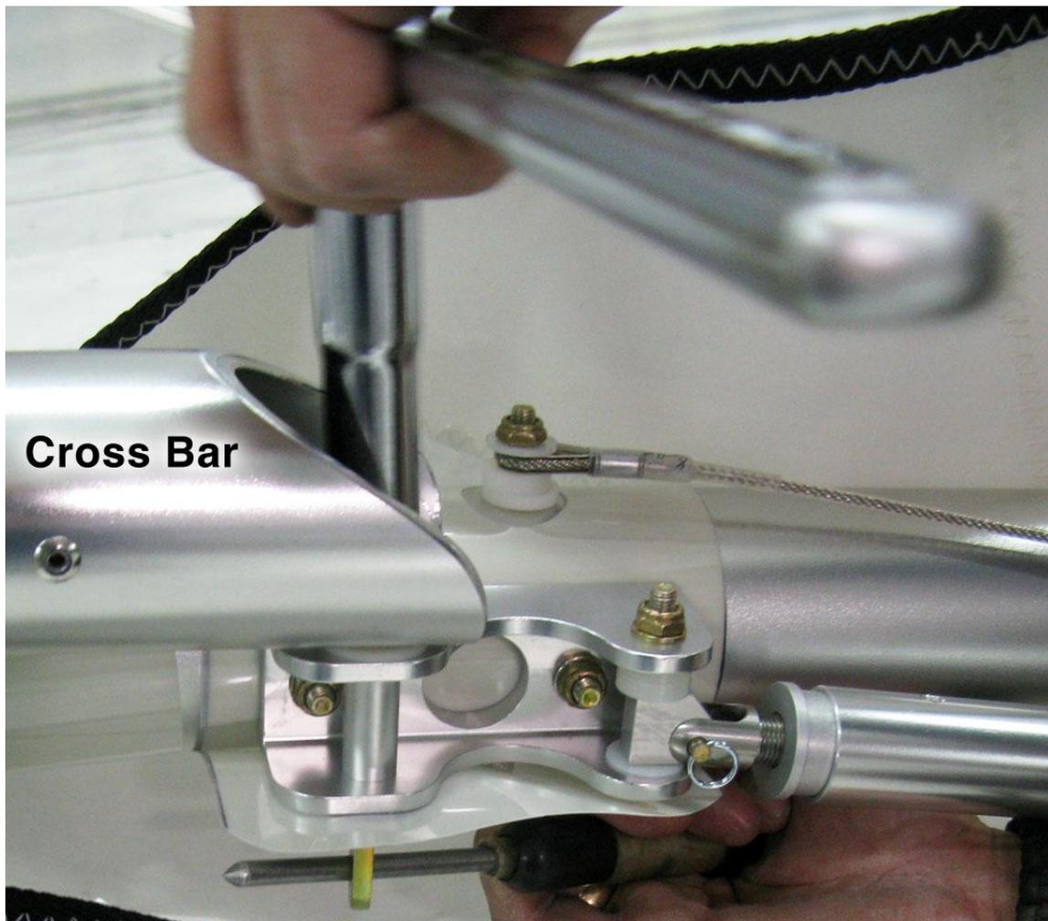
**Photo: Raising the nose of the wing and extending the Base Tube**
