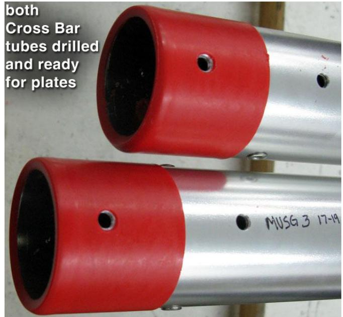
4. Prepare the center plates to be attached to cross bar tubes by using the Schematic Diagram labeled “Cross Bar Center Junctions” to arrange the layout of plates with bolts, half-spacers, washers, and Nylock nuts.
