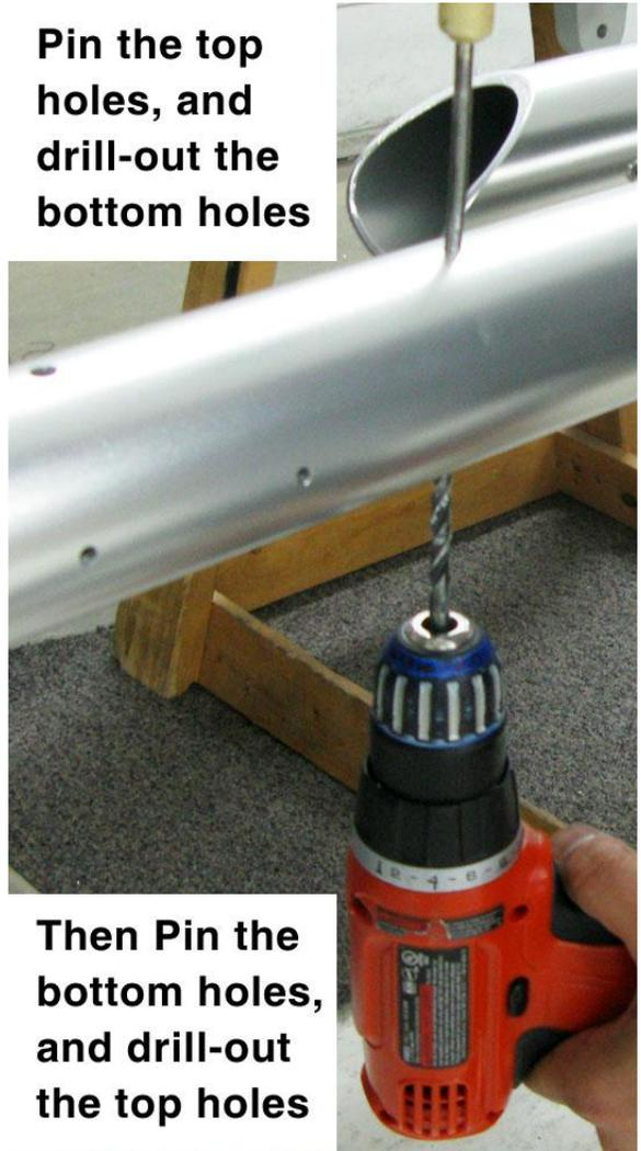
**Then Pin the bottom holes, and drill-out the top holes**
