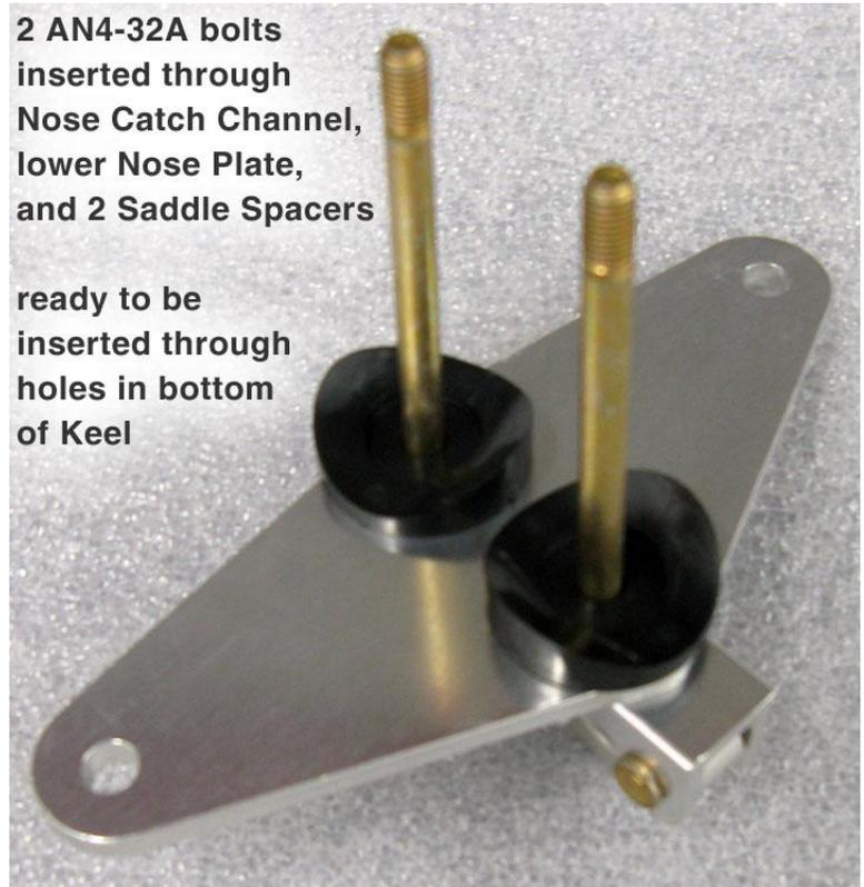
Photo: Attaching Top Nose Plate to Keel
