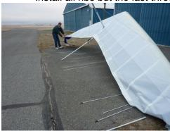
6. <u>FIND THE CROSS TUBE TENSION</u> cable retrieve line and pull it through the keel pocket till you can get the black webbing handle. Pull the shackle back and latch into the spring catch.
