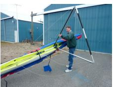
2. <u>ROLL THE WING OVER</u> stand wing on the control frame. Check to make sure the lower side wire cable thimbles have not turned 180 degs and will get kinked if tensioned. (do not attach the lower front wires at this time) FIG
