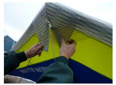
13. <u>ROTATE THE SPROGS</u> into position and zip up the sail. Sprog sets between the 1" webbing strap and the zipper.
