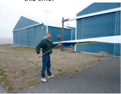
10. <u>INSTALL THE NOSE BATTENS</u> (tail end first) from the nose of the glider, now seat the front end of the rib on the standoffs just in front of the nose plate. Nose ribs can stay in the glider if you wish by taking them off the stand offs at the nose when packing up.
