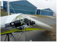
11. <u>ATTACH THE FRONT FLYING WIRES</u> at the nose plate area by slipping the ring around the nose spring catch. **ENSURE THAT THE SPRING IS PROPERLY SETTED** so it is pushing up on the top of the latch.
