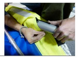
Install the base tube on the VG side (right side) of the control frame. You are now ready to set up your glider. If you have the Fast foil control frame you will put the BT on as you set up.
