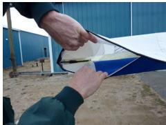
9. <u>INSTALL THE LAST THREE CURVED</u> ribs and secures all the flip tip tension levers at this time.
