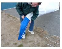
• <u>FOLDING WINGS IN</u>, always fold the wings together symmetrically, bringing both leading edges back together at the same time. An alternative to having someone help bringing in both leading edges at once, is to bring in one a bit, then the other a bit more, in three to four incremental steps. If you meet resistance folding in the wings, check that the cross tube tensioning line or cable are free to run forward through the cable hole center of the sail.
