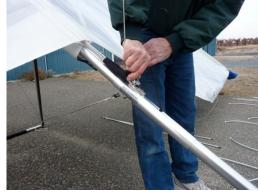
7. HOOK THE LOWER REAR TOP WIRE triangle ring into the same spring catch.
