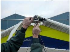
12. <u>INSTALL THE GLIDER'S NOSE CONE</u> starting with the two top velcro tabs and gently pulling the shroud down and around the nose plate to connect the two bottom velcros of the nose cone to its corresponding velcro on the under-surface.
