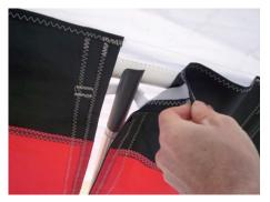
14. <u>INSTALL THE UNDER SURFACE</u> ribs from longest to shortest. Make sure the back ends are inserted back into the slot at the rear.
